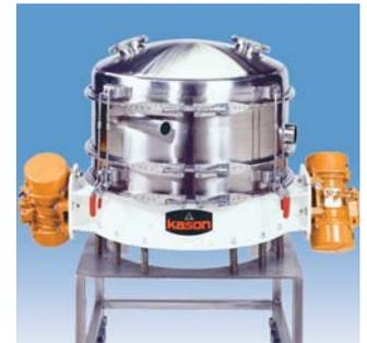
**PNEUMATI-SIFTER/FLO-THRU Dual-Screen Ultra-High-Capacity Separator**
